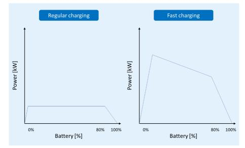
Figure 3: The charging curve of an AC and DC charging station.
