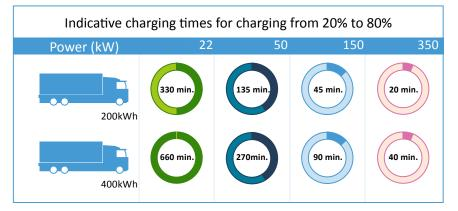
Figure 1 shows several representative charging times for an electric truck with a 200 and 400 kWh battery pack. Future developments relating to charging speeds are discussed briefly in §2.8.
